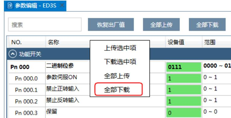
The screenshot shows a table of parameters under the heading '功能开关' (Function Switches). The table has columns for NO., Name, Device Value, and Range. A context menu is open over the row for Pn 000.2, with the '全部下载' (All Download) option highlighted in red.
