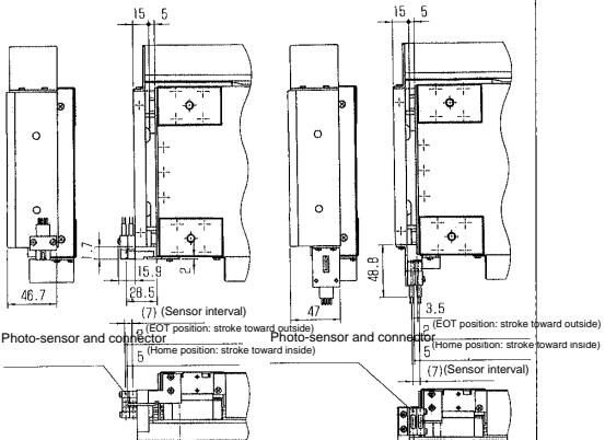
Photo-sensor: EE-SX670A (Omron)
