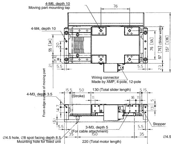
Unit in figure: mm
